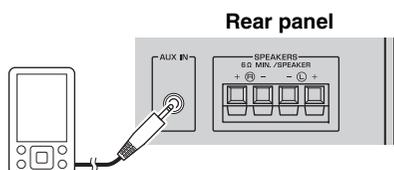
Using a commercially available 3.5 mm stereo mini-plug cable, connect your external device to the AUX jack on the rear panel of this unit.
