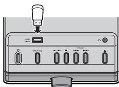
Connect your USB device to the USB port on the top panel. For details on playable files, refer to "NOTES ON DISCS AND USB DEVICES" (P. 21).
