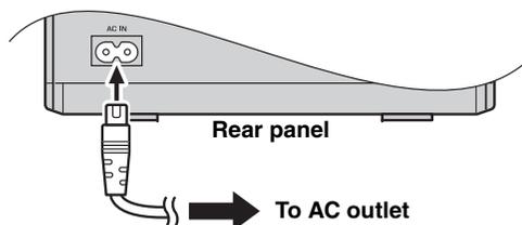
When you've completed all connections, connect the supplied power cable to AC IN, and then connect the plug of the cable to an AC outlet.
