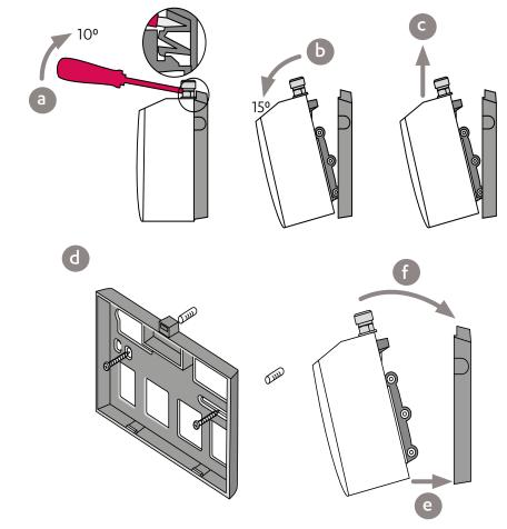
**Note** Take care not to break the clips when removing or installing the Booster.
