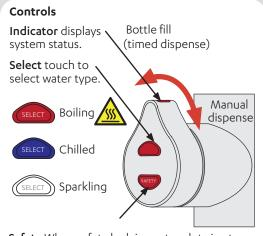
**Safety** When safety lock is on, touch twice to flash. Turn to dispense boiling water.
