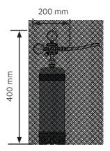
Secure cylinder vertically to a robust surface with the hook & loop strap and
