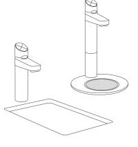
HydroTap Elite Plus can be installed over sink or optional font
