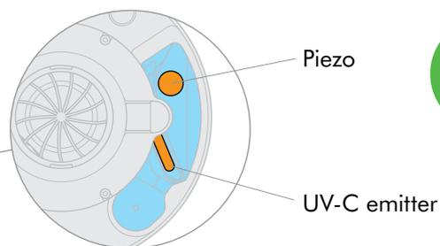
dishwasher. Fill the trough with the recommended acid citric solution until the UV-C emitter and piezo are submerged. Leave for 15 minutes. Drain, rinse and wipe over all surfaces. Repeat if necessary.
