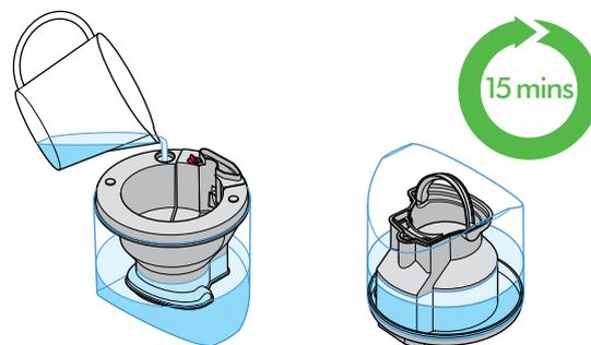
Pour in the recommended citric acid solution. Replace the cap and shake tank for 30 seconds. Then leave to stand. After 15 minutes, empty the tank. Rinse and wipe over all surfaces. Repeat if necessary.
