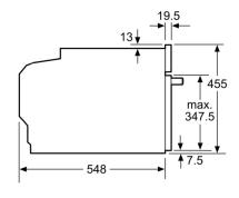
measurements in mm
