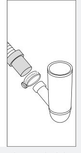
The drainage hose can also be connected to a connection nipple on the sink unit's water trap. The connection nipple must have an internal diameter of at least 14 mm.
