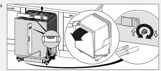
5 Adjust the front feet by turning them clockwise to raise and anticlockwise to lower the dishwasher.
