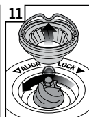
Push upper burr firmly into position
