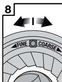
Move adjustable top burr, 1 number, coarser or finer
