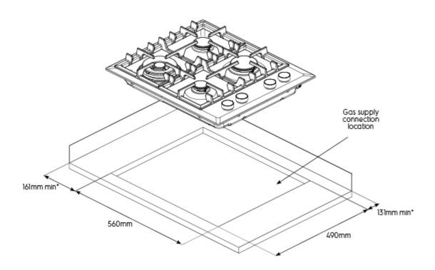
\*To combustible surface (dimension is not relevant if the adjacent surface is non-combustible).
