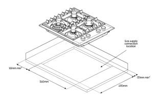
\*To combustible surface (dimension is not relevant if the adjacent surface is non-combustible).
