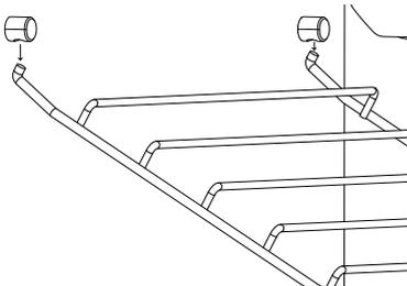
Swing the bottom of the side rack up towards the center of the oven until it is almost horizontal. Slide the prongs at the top out of the mounting slots.
