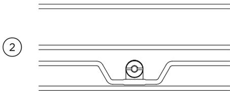
Ensure the prongs are fully inserted into the slots before lowering the side rack carefully and refit the fixing nut. It is important to ensure the tab behind the fixing nut sit flush against the wall. A coin may be used to tighten.
