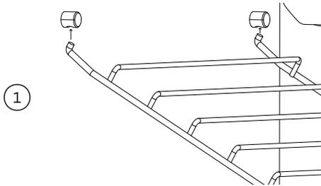
Supporting the side rack from underneath, hold it almost horizontally and locate the prongs into the mounting slots.
