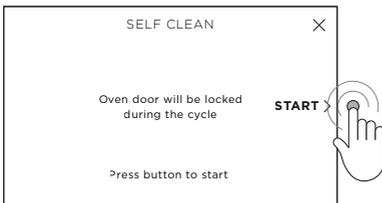
Press the middle button to the right of the screen to start the clean cycle.
