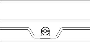
Unscrew the fixing nut holding the side rack in position. A coin may be used to loosen.
