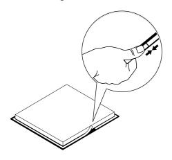
Assemble spring clips as shown, to support unit in benchtop.
