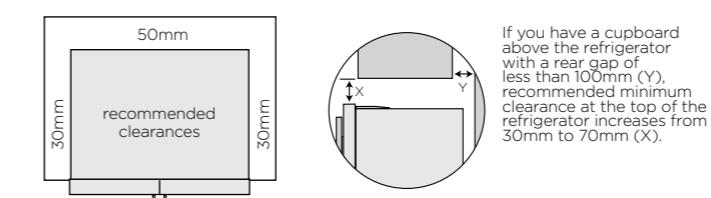
If you have a cupboard above the refrigerator with a rear gap of less than 100mm (Y), recommended minimum clearance at the top of the refrigerator increases from 30mm to 70mm (X).
