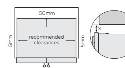
If you have a cupboard above the refrigerator with a rear gap of less than 100mm (Y), recommended minimum clearance at the top of the refrigerator increases from 30mm to 70mm (X).
