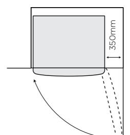
When positioned in a corner, the clearance must be at least 350mm on the hinge side to allow the door to open smoothly so that bins and shelves can be removed easily.
