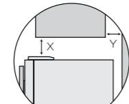
If you have a cupboard above the refrigerator with a rear gap of less than 100mm (Y), recommended minimum clearance at the top of the refrigerator increases from 50mm to 100mm (X).
