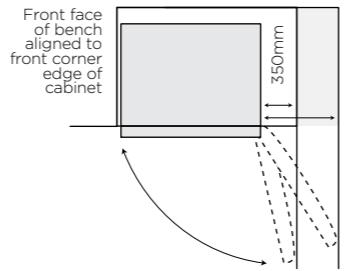
Front face of bench aligned to front corner edge of cabinet
